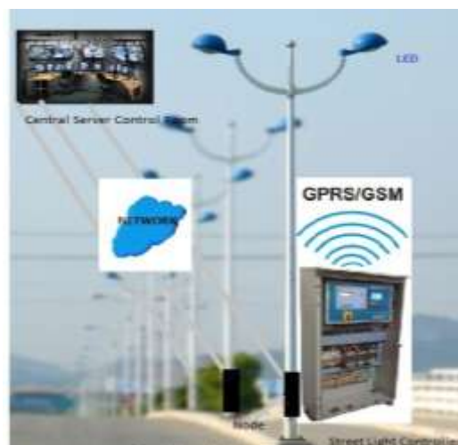
Figure 4: Intelligent Street Lighting Sys
