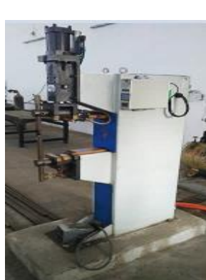
Fig. 2 Spot welder model SS-35-450
