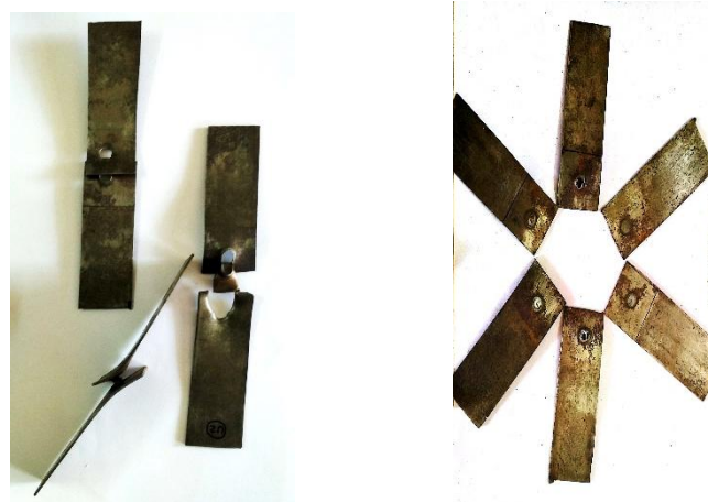
Fig. 10 (a) Pull out failure (b) Interfacial failure
