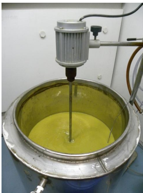
Figure 2: Experimental set up for dissolution of uranium metal chips using sodium hypochlorite solution, Batch Size: 4 Kg.
