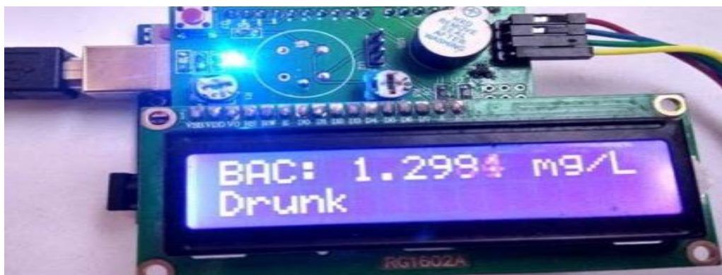
Fig. 11. Output of the MQ-3 sensor module showing on the LCD with a failed breathalyzer test
