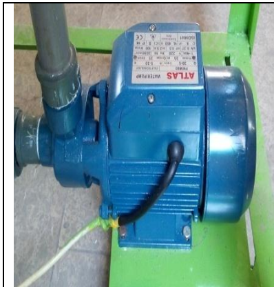
a). 0.5HP water pump
