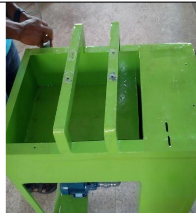
b). Turbine frame with water tank
