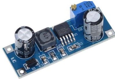
Figure 8: 7W Bulk converter.
