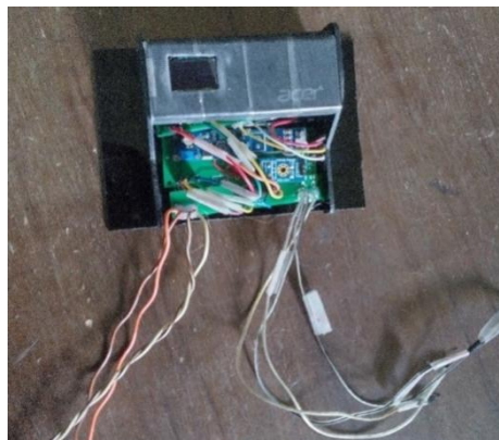
Figure 11: Constructed ESP 32 based weather monitoring system
