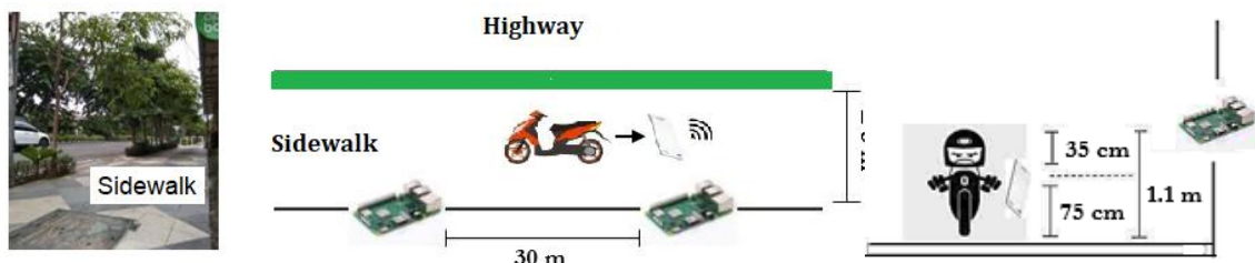
Fig.2. System implementation on sidewalks.
