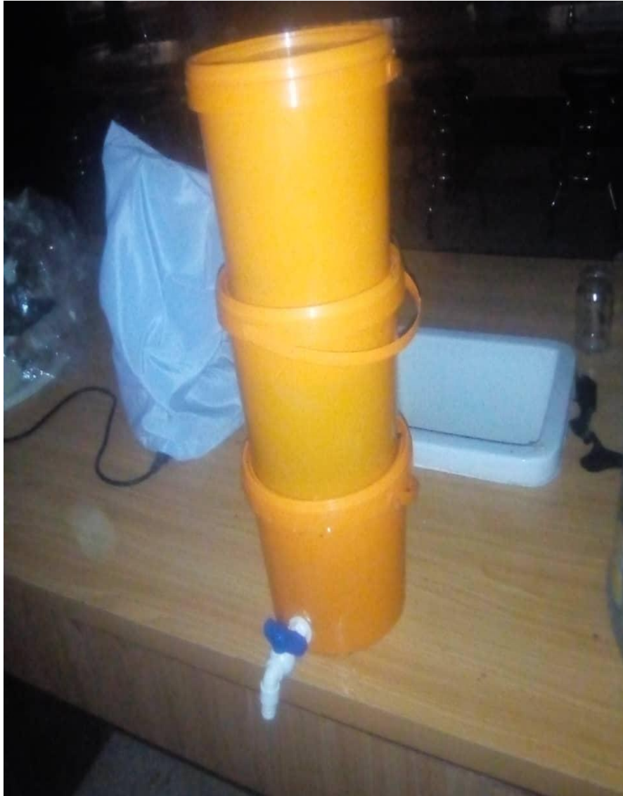
Figure 1. Shows the constructed portable water treatment plant, with three layers of horizontal frames. Tank A, tank B, and tank C layers has the same size. The layers of the tanks are all plastic bucket. Firstly, there is a PVC pipe which connect tank A to the tank B which water pass through. Then there is a micro filter attached inside the tank C which the water passes through. After that a tap was inserted through an open hole in the bottom layer / tank C.
