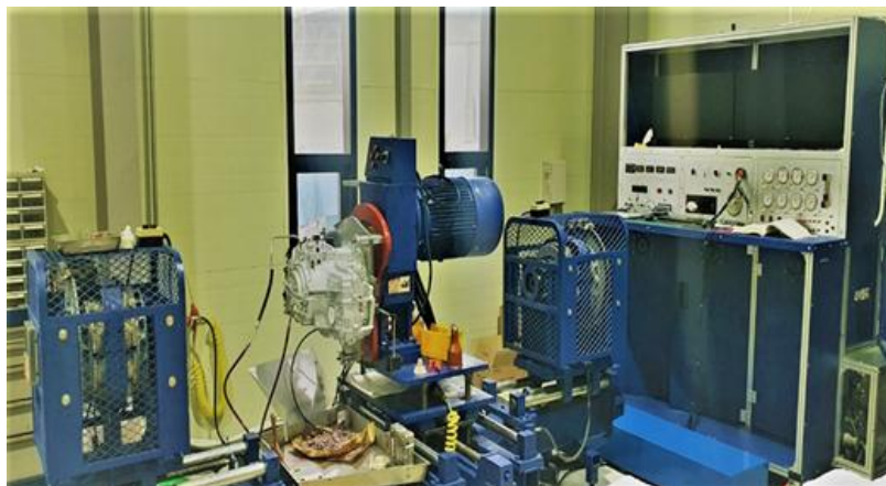
Figure 1. Performance demonstration test bed for remanufactured CVT
