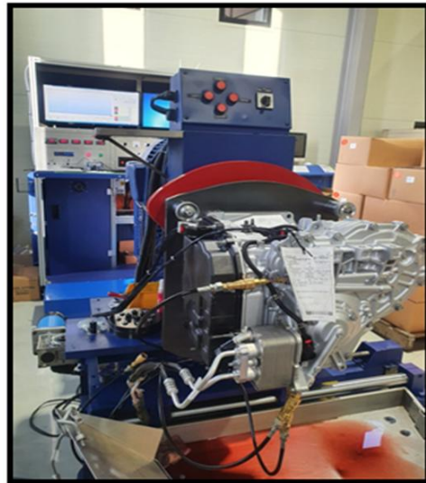
Figure 3. Remanufactured CVT mounting on the Performance demonstration test bed
