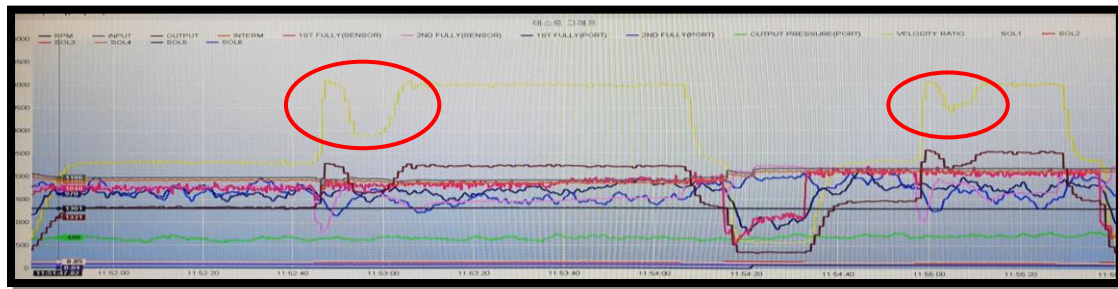
Figure 6. The experimental graph of the gear ratio change according to the change of the primary and secondary pulleys
