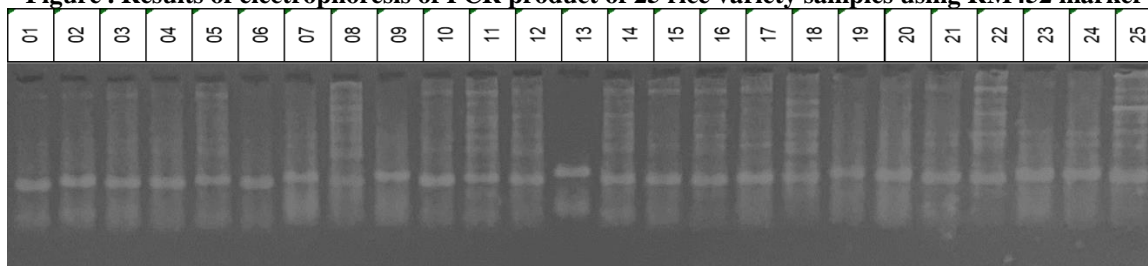
Figure . Results of electrophoresis of PCR product of 25 rice variety samples using OSR13 marker
