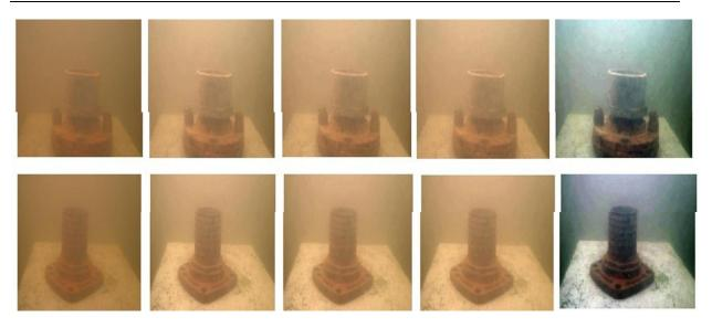
Fig: First column: original image, second column: after homomorphic filtering, third column: after wavelet denoising, fourth column: after Bilateral filtering, last column: after contrast equalization
