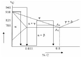
Fig. 5: Schematic heat treatment diagram: As received and intermediate quenching process  $\alpha$  Ferrite,  $\beta$ : Cementite,  $\gamma$ : Austenite
