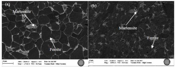
Fig. 6: Optical micrograph of (a) DPS-780°C (b) DPS -825°C
