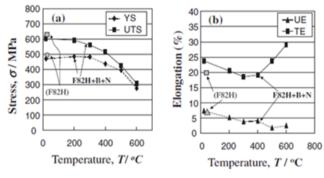
Fig. 8, 9: Tensile properties of F82H+60ppm+200ppm N steel
