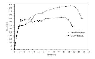
Fig. 3: Stress versus strain curve for tempered and control specimen.
