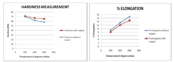
Fig. 7: Hardness and Elongation measurement
