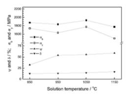
Fig. 13: Effect of ST temperature on tensile properties after ST+CT+AT at 535°C for 4 h.
