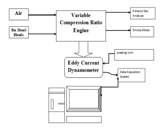
Fig4: Block diagram of Experimental Procedure
