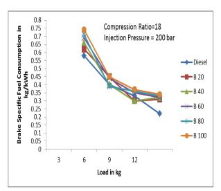
Load v/s Brake Specific Fuel Consumption
