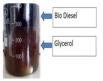
Fig2: Transerterified mixture
