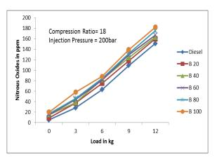
The nitrous oxides (NOx) emission is a function of combustion temperature and the combustion chamber [18]. The relationship of load and nitrous Oxides emission is linear increasing in manner. The Nitrous oxides emission of B 100 is found is highest and lowest is diesel. NOx emission of B100 increased by 36%. B 20 by 13% when compared with mineral diesel.
