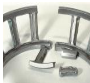
Figure7. Failure of cage
