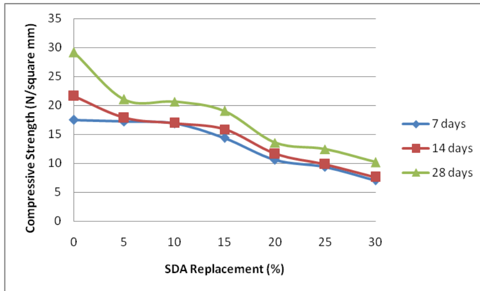
Figure 2: Effect of SDA content on Compressive Strength of concrete at different curing age
