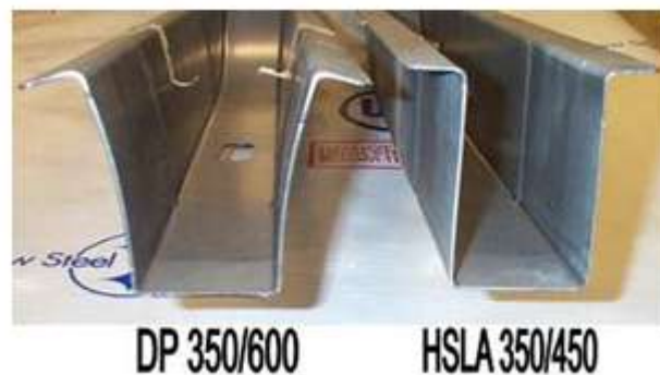
Figure 7. Elevated springback issues for DP steels compared to HSLA steel [26].
