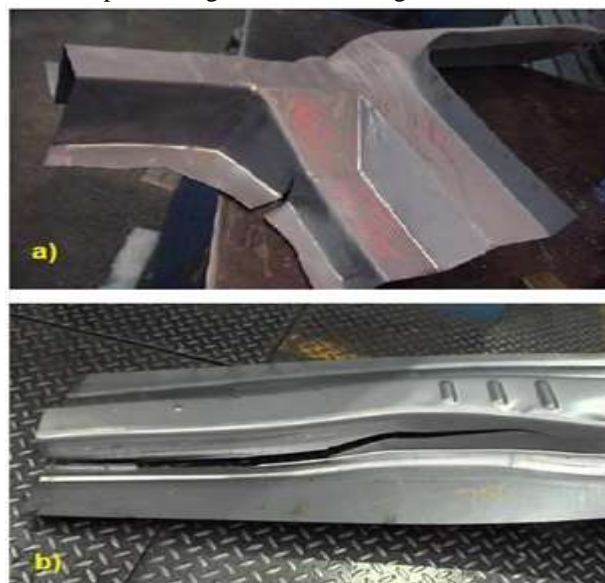
Figure 8. Different failure modes for AHSS parts a) edge stretch cracking, b) stretch bending fracture of DP 780 [36]
