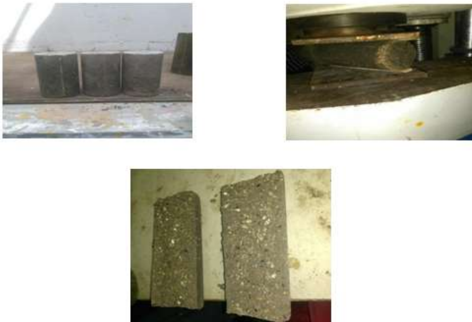
Figure 2 Split Tensile strength testing on with fibre cement vermiculite cylinders
