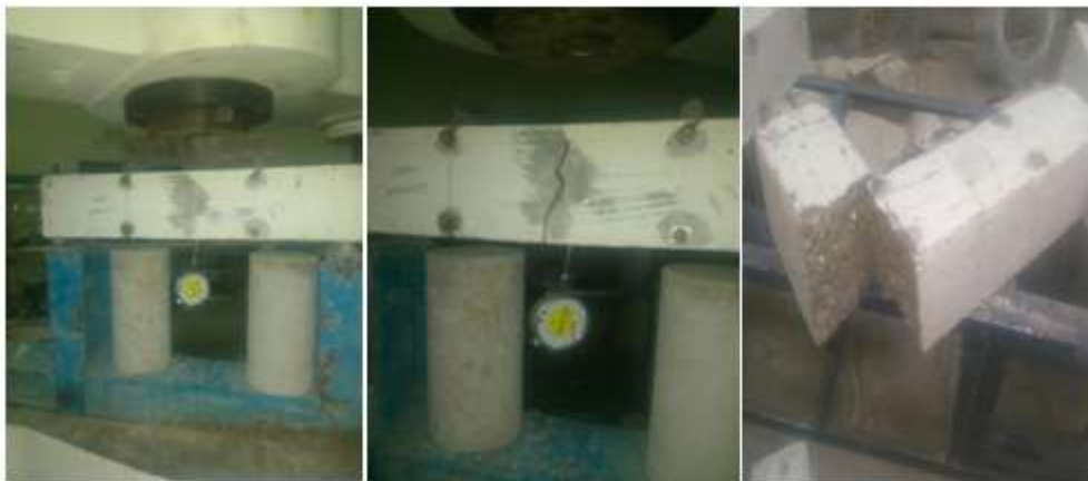
Figure 3 Flexural strength testing on without fibre cement vermiculite slab
