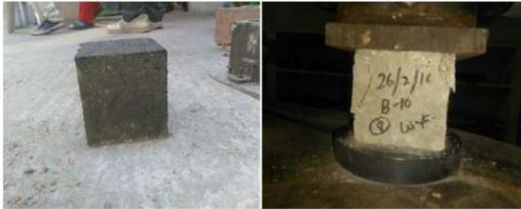
Figure 1 Compressive strength testing on with fibre cement vermiculite cubes.
