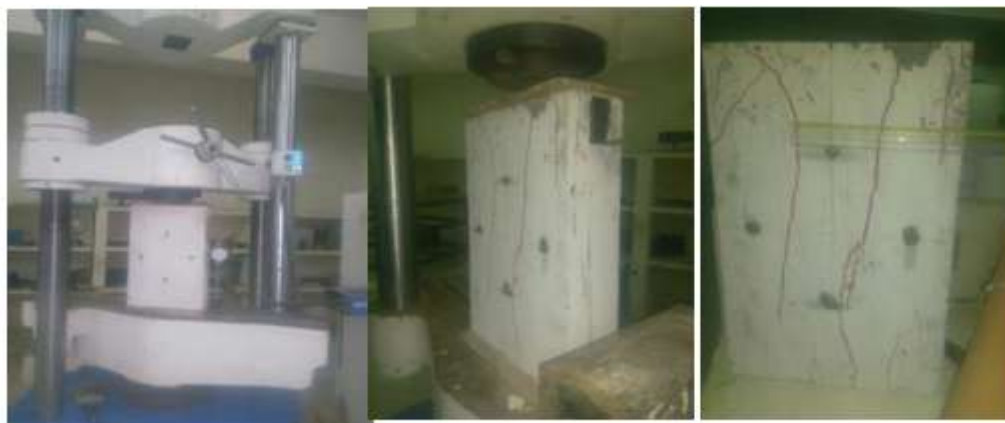
Figure 4 Uniaxial compression test on Ferro-vermiculite panel – 300x 450 mm
