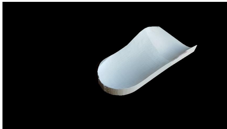
Figure 6. Fresh insole model after printing process
