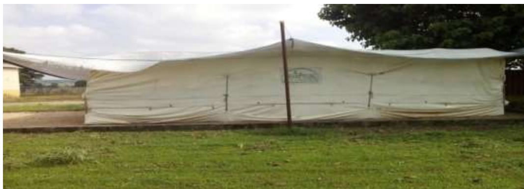
Plate 2: An assembled grain storage Cocoon in National Strategic Food Reserve Silo Complex, Minna, Nigeria.
