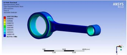
Fig.7. Equivalent Strain in Aluminum Alloy 6061 connecting rod
