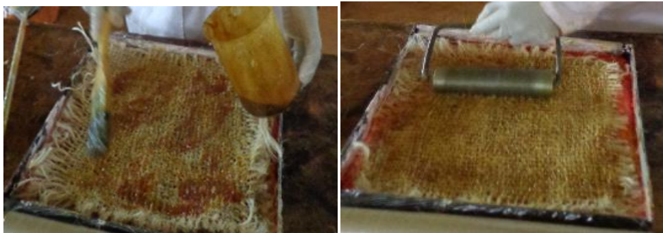
Figure 1: Application and squeezing the matrix into the fibres
