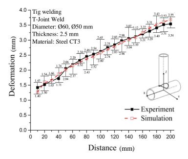
Figure 5.Deformation of a 2.5-mm-thick pipe.
