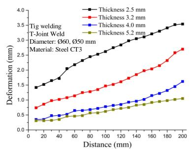
Figure 4. Comparison of pipe deformations for different pipe thicknesses.
