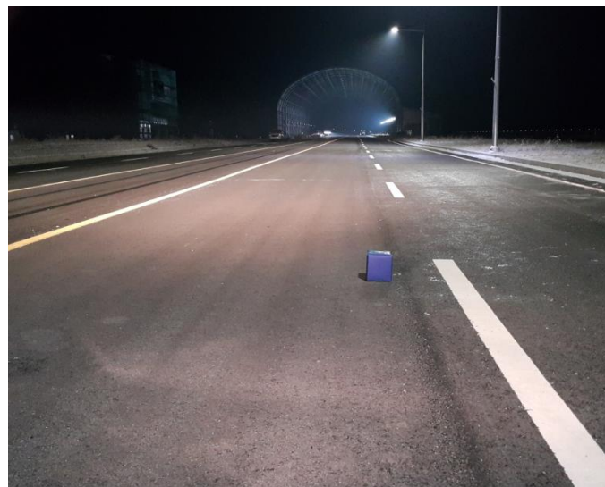
Fig:6 Obstacles (pole lighting zone, reflectivity 10%)
