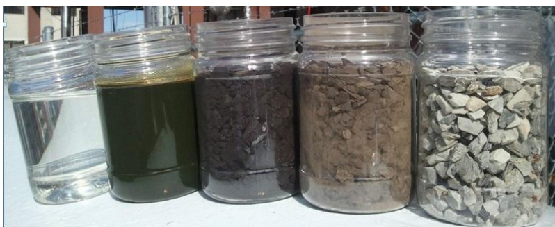
Figure 8 – right to left: raw oil shale, low temp spent shale, high temp spent shale, shale oil, refined oil
