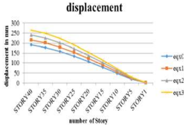
Figure-2: Displacement for static case along x direction with p-delta.
