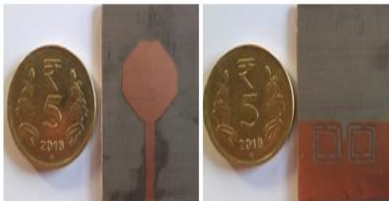
Fig. 4 (a) Fabricated monopole antenna (Front and Back view)
