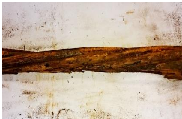
Figure 2.1 PC steel bar after accelerated corrosion for 8 days.
