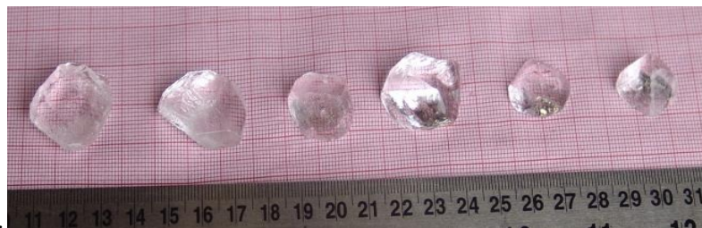
Figure 1: Photograph showing the undoped and ADP doped DSHP crystals grown [From left are : 0.0 (undoped DSHP), 0.2, 0.4, 0.6, 0.8 and 1.0 mole% ADP doped]
