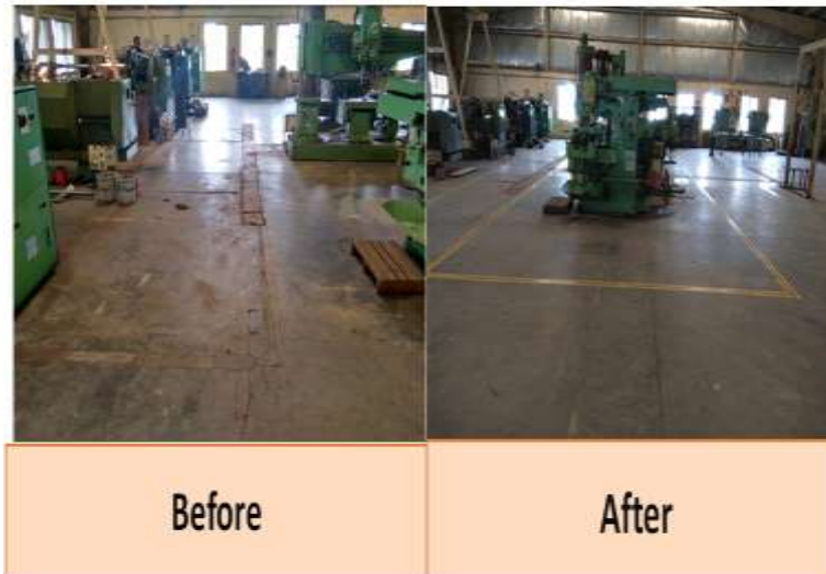
FIG 13: Photograph before and after (Marking of Work area)
