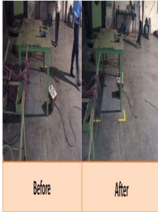
FIG17: Photograph before and after (proper area marking)
