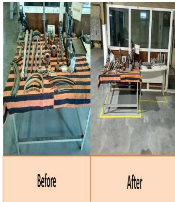
FIG 14: Photograph before and after (Marking of area)
