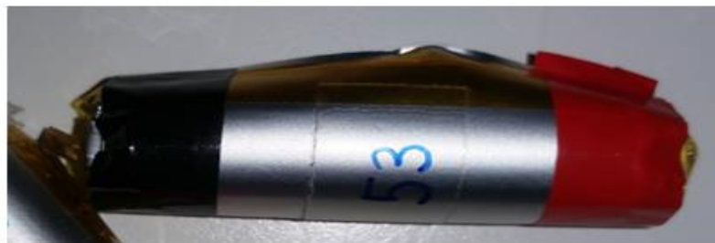
Figure 9: LIR13450 bloated cell after the cyclic test of CCCV charging in 30 minutes.
