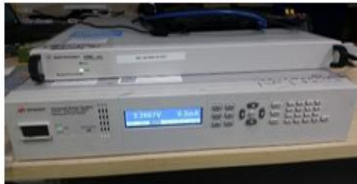
Figure 3: KEYSIGHT, Power Supply with max Current of 50A
