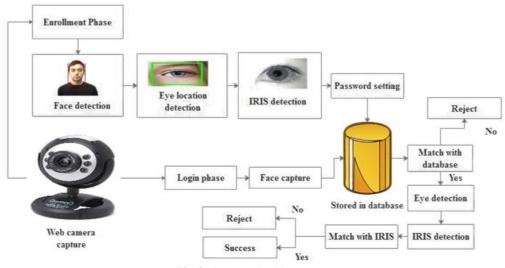
Fig 2: System Architecture
