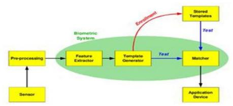
Fig 1: Block Diagram Of Biometric System
