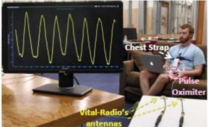
Fig. 6: Experiment For Vital Sign Monitoring. [15]
