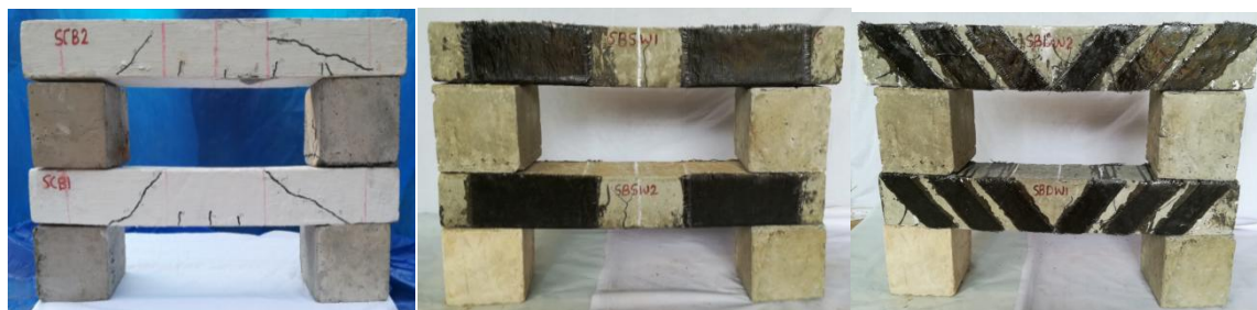
(a) Control beam (b) Shear zone wrapped beam (c) Diagonal wrapped beam Fig. 6 Failure pattern
