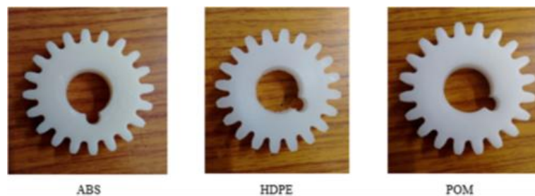
Fig 2. Injection moulded gears [13]
