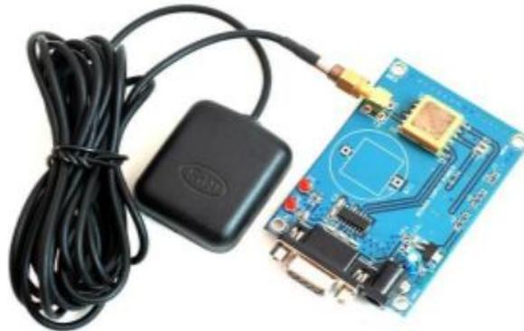
The Global Positioning System (Gps) Is A Global Navigation Satellite System That Provides Location And Time Information In All Weather Conditions. Gps Satellites Transmit Signal Information To Earth. This Signal Information Is Received By The Gps Antenna In Order To Measure The User'S Correct Position.
