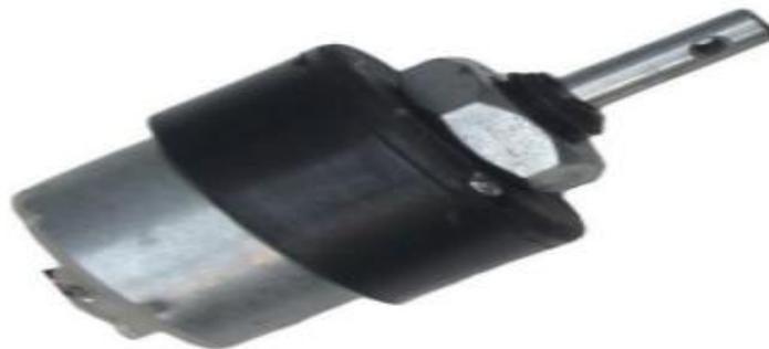
Geared Dc Motors Can Be Defined As A N Extension Of Dc Motors A Geared Dc Motor Has A Gear Assembly Attached To The Motor. The Speed Of Motor Is Counted In Terms Of Rotations Of The Shaft Per Minute And Is Termed As Rpm .The Gear Assembly Helps In Increasing The Torque And Reducing The Speed.
