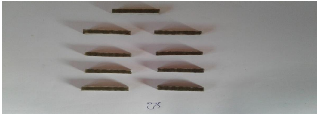
Fig 1.8 Specimens of S2 composite material for pin-on-disc test
