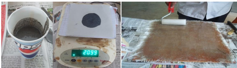
Fig 1.2 Mixture of matrix material with varies wt% of fillers Fig 1.3 Fabrication by hand lay-up method
