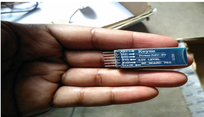
Fig.8 Bluetooth module device to transfer data signals from analog to digital from the device to smart phone
