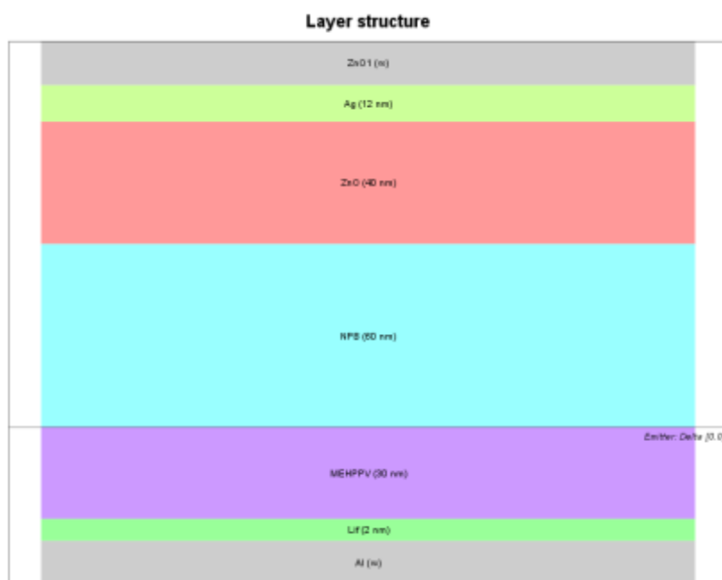
Fig 5: The structure of the OLED used ZnO/Ag/ZnO as anode
