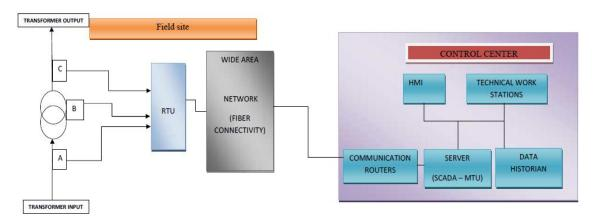
The figure above shows a block diagram of transformer monitoring model. The figure below shows a block diagram of stage of implementation model.
