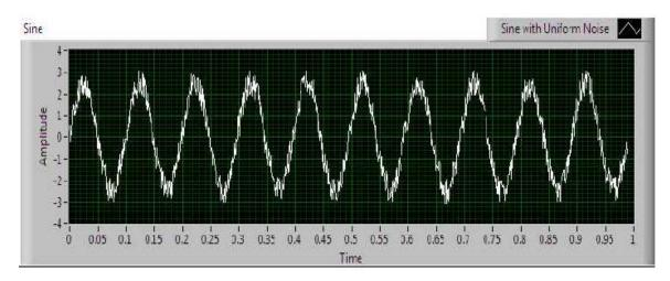
When the transformer is powered the secondary output voltage is sensed and acquired by the DAQ taking in a maximum of 5V varying from an integer 1 to 5. Any superimposed noise voltage appears above the true 5V secondary output. When a value above 5 is recorded an alarm warning will be enabled indicating unhealthy transformer. This is showed below; front panel (i) and (ii).
