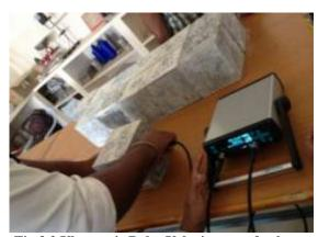
Fig.3.2 Ultrasonic Pulse Velocity test of cubes
