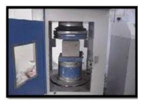
Fig.3.1 compressive strength of cubes
