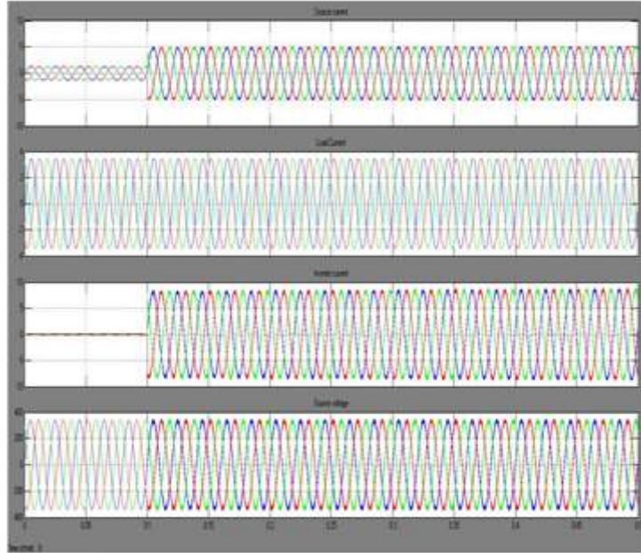
Figure.12. Simulation results of Un-balanced Linear load (a) Source voltage(b)source current(c) load current(d) Source Current SRM Motor connected to the proposed Circuit.
