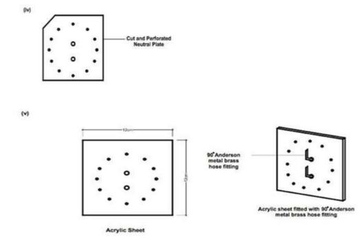
Figure 1. Cuts components of HHO generator
