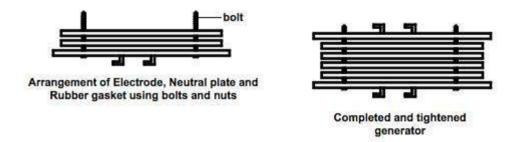
Figure 2. The step-wisearrangement of the oxyhydrogen generator electrode plates
