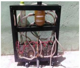
Figure 3. Front view of the oxyhydrogen generator
