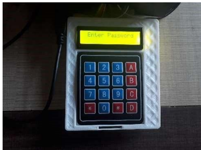
Fig 6 Keypad based ignition control
