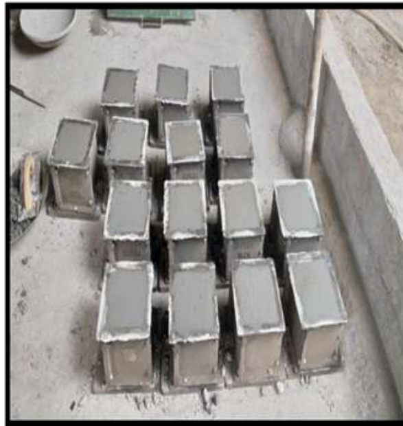
Figure 3: Casting of cubes
