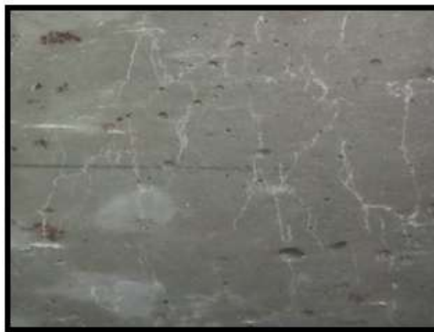
Figure 6 : Healed cracks of Bacterial Beads&Silica gel.
