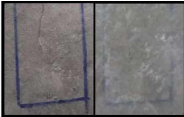
Figure 5: Healed crack of bacterial solution.
