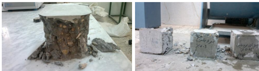
Fig 1: Cubes after strength test
