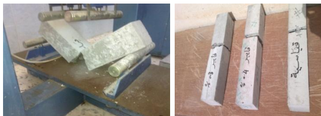
Fig 3: The bending resistance test after 28 days
