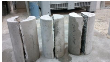
Fig 2: The tensile strength test after 28 days
