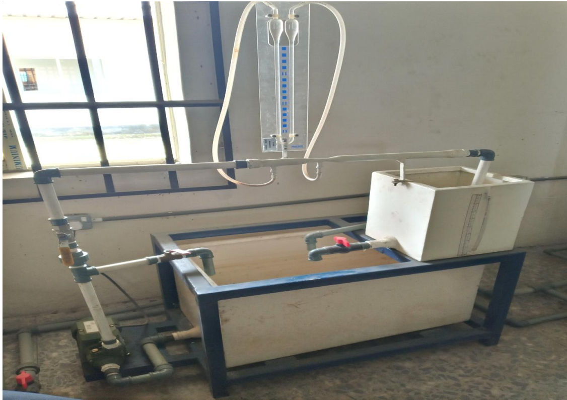
Figure 1.2: Shows the manufactured Venturimeter flow rig being integrated alongside other fluid mechanics equipment in the fluid mechanics laboratory in AKSU, Nigeria
