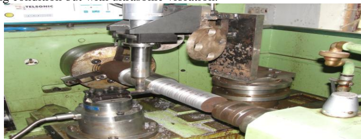
Figure4. Work piece preparation in UAT using lathe (HMT Model NH 26).
