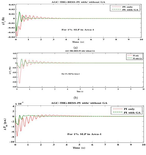
(c) Fig 6(a, b, c) BESS with AGC- THG- PI with/ without GA for 1% SLP in Area -1
