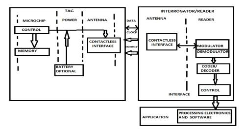
Fig.1 shows the Block Diagram Representation of RFID System Components
